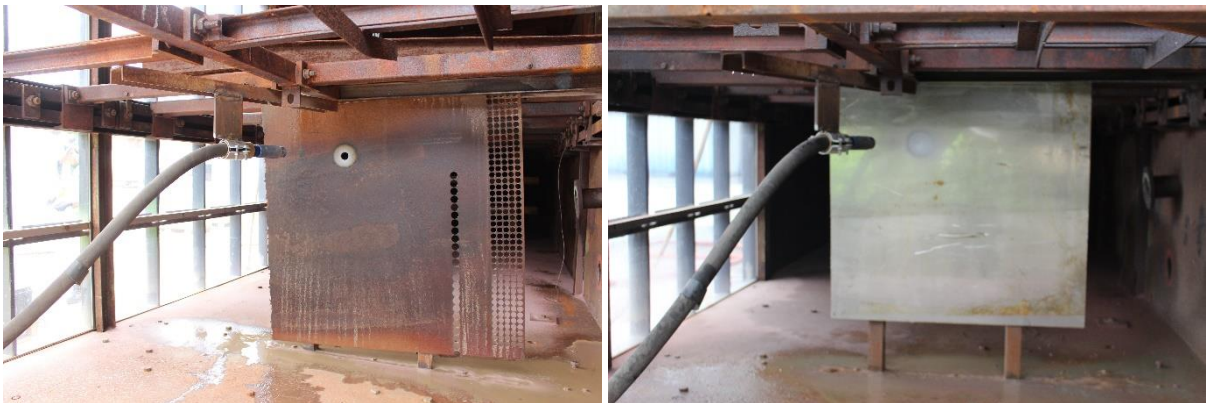
Figure 2-9 Pictures of the test setup with the nozzle blasting on a steel and aluminum plate.
