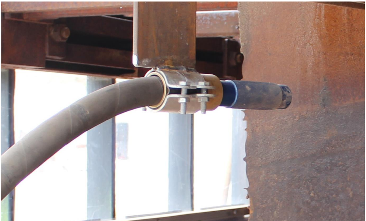
Figure 2-5 Nozzle mounted inside the testing vessel. The nozzle was electrical isolated from the steel using a rubber seal.
